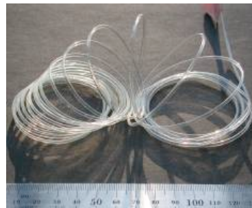
Fig. 1: Extruded microtubing (2.7g) obtained with a draw-down of around one.
